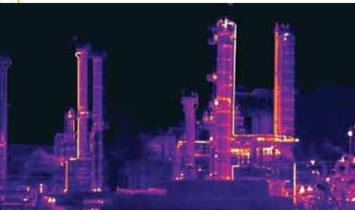
*Optical gas imaging cameras give you the power to spot invisible gases as they escape, so you can find fugitive emissions faster and more reliably than with sniffer detectors. With a FLIR GF-Series camera, you can document gas leaks that lead to lost product, lost revenue, fines, and safety hazards.*
