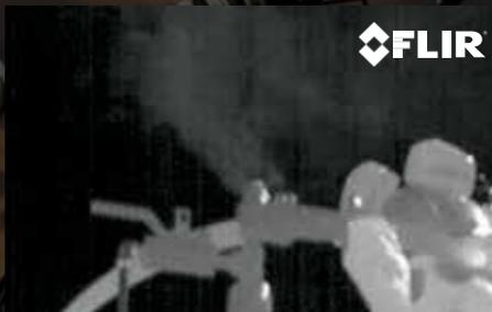
COMMON SF<sub>6</sub> PLUMBING LEAK
