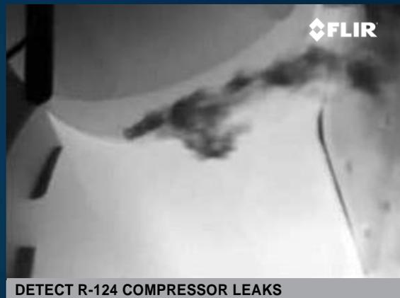
DETECT R-124 COMPRESSOR LEAKS
